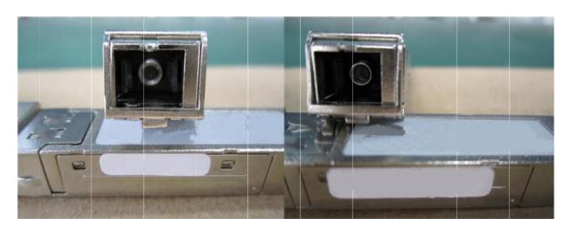
Those two SC slots from the twins. One is OBB24531A, SFP Bi-Di transceiver, 1.25G TX1490/Rx1550nm 100KM SC DDMI  $0\sim70^{\circ}$ C +3.3V, another one is OBB25431A, SFP Bi-Di transceiver, 1.25G TX1550/Rx1490nm 100KM SC DDMI  $0\sim70^{\circ}$ C +3.3V, they look like
